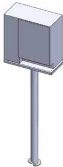
Helical Pile with utility cabinet installed
