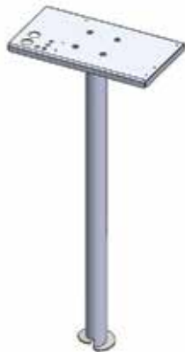
Helical Pile with Custom Adapter Plate
